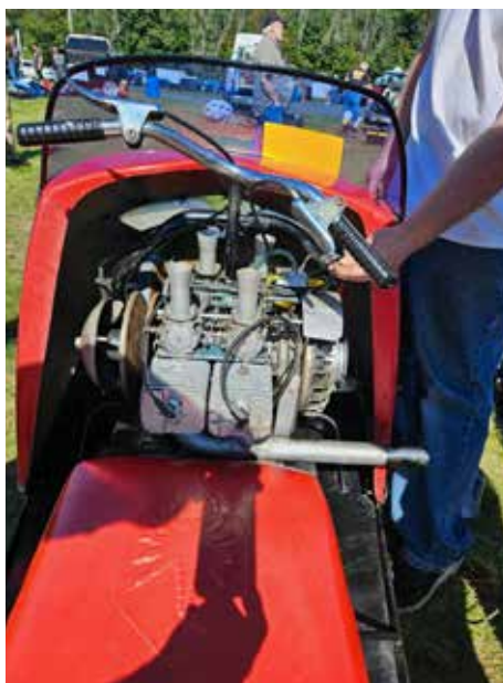
Nick Ruddy's Scorpion stinger with a four cylinder, four carb aircraft engine
