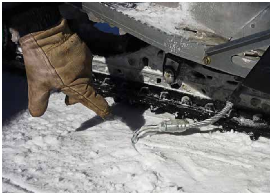
Once deployed, the Duraflex scratchers spray snow into the suspension.
